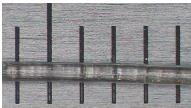
Figure 1. Photograph of a low doped (0.5 mol%) \text{CaTa}_2\text{O}_6:\text{Nd}^{3+} single crystal fibre grown by LHPG. The scale is in millimetres.
